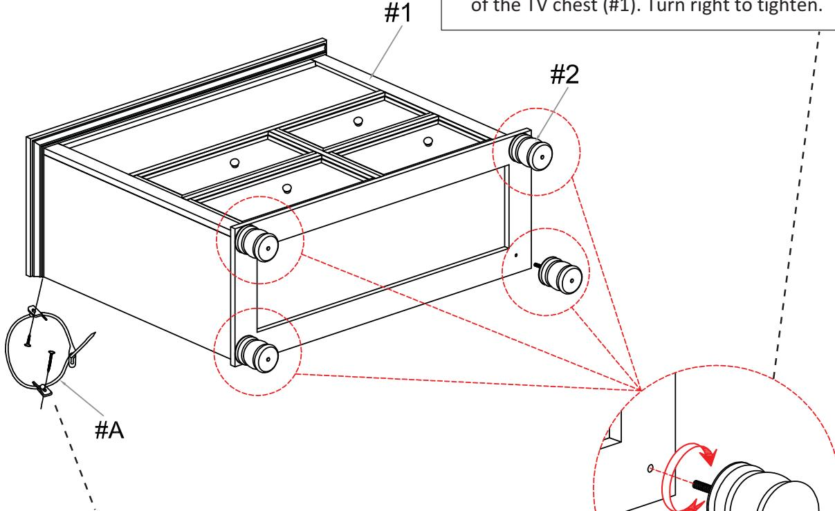
2. Align a bracket along the tipping restraint to a wall then insert a screw and use a power tool to secure. After that place the TV chest in position and align the other bracket to the back of the TV chest. Secure and tighten strap accordingly.
