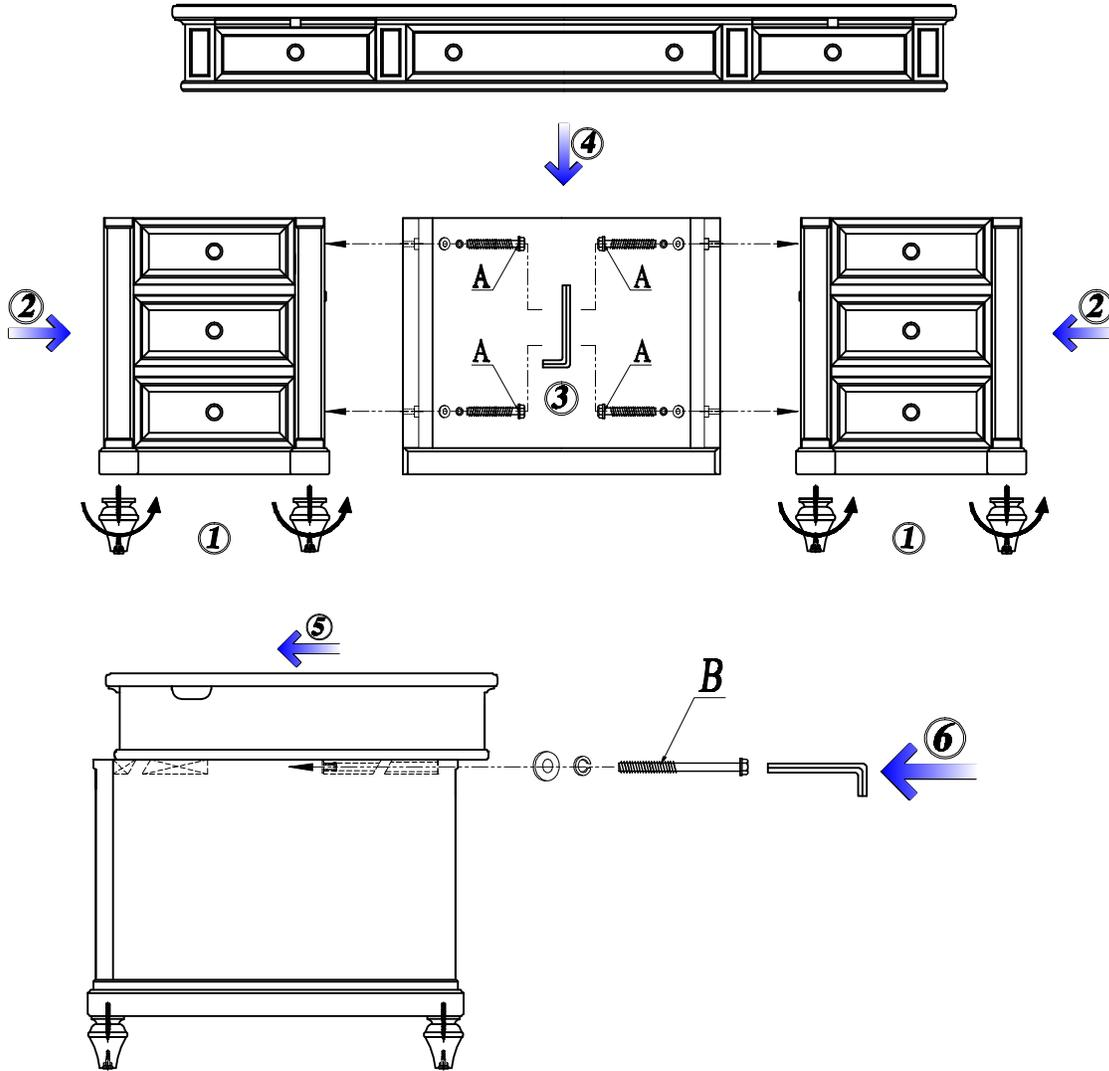
1. Place the top upside down on soft surface to prevent scratching, and rotate the bun feet to be tightened by hands.
