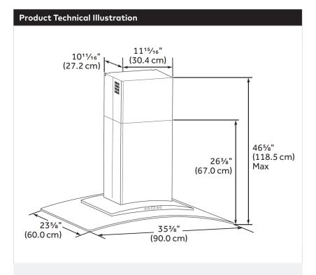
**Note:** The vent hood must be installed 24" min. above electric cooktop surface and 30" min. above gas cooktop surface.
