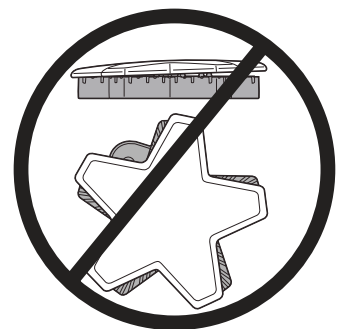
Incorrect burner cap
