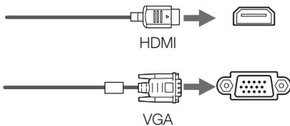
**Note:** If you are connecting via HDMI, use the **HDMI1** or **HDMI2** port on the projector. For a VGA connection, use the **Computer1** port. To use other ports on the projector, see the online *User's Guide*.
