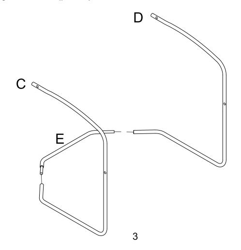
Step 3. Attach support legs (parts C & D) to chair back (part A) and chair seat (part B) using long bolts (part #2), Round Plastic Washer (part #8), and flat washers (part #4), plastic washers (part #5), nuts (part #3), wrench (part #6) and allen wrench (part #7).
