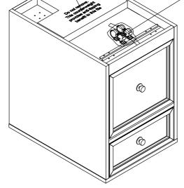
The above diagram shows a counter weight placed under the bottom of the fle cablnet. Do not remove this weight as it will greatly reduce the chance of tip over.
