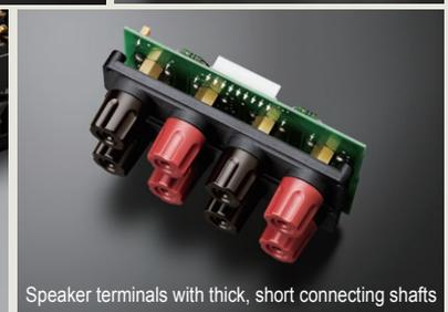
Speaker terminals with thick, short connecting shafts
