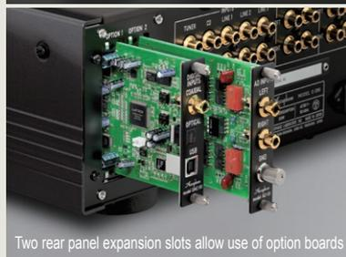
Two rear panel expansion slots allow use of option boards
