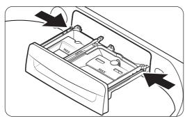
**2.** To remove, pull the detergent drawer while pushing the ends of each side in.
