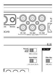
If you wish to send six discrete channels into the M600/6, simply use all six inputs and set the "Input Mode" switch in the "6 Ch." position.
