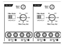
1) "Filter Mode" Control: The M600/6 employs a 12dB per octave filter for each pair of channels (one filter for channels 1&2, another filter for channels 3&4 and a third filter for channels 5&6). Each of these filters can be configured independently into one of two filter types or defeated completely by way of the three-position "Filter Mode" switches:
