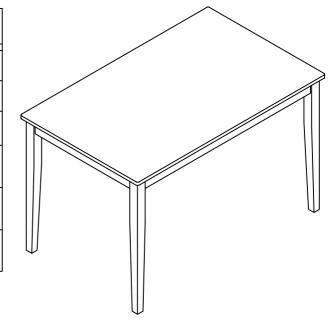
Important note: Place all wooden parts on a clean and smooth surface such as a rug or carpet to avoid the parts from being scratched. Affix the table legs (B) to the corner block with hex crew (C) spring washer (D). And flat washer (E). Then tighten the hex screw (C). by using the alien key (F).
