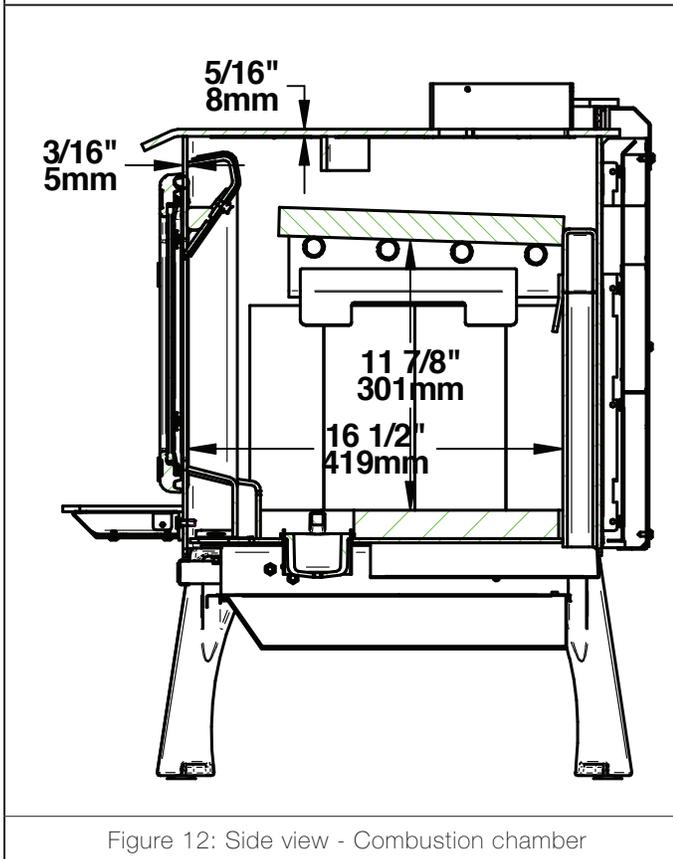
Figure 12: Side view - Combustion chamber
