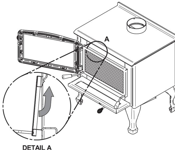
3. Lean the upper part of the fire screen against the top door opening making sure to stow the top fire screen brackets behind the primary air deflector.
