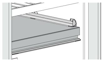
Pull out the serving shelf a little (1), lift the front upwards (2) to release the magnetic connection, and pull it out forward (3).
