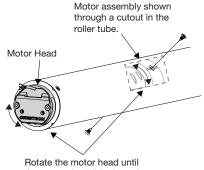
Rotate the motor head until the groove is visible through the screw hole, and then install the screws.
