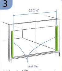
Add vertical fillers to the opening width. The width of the opening should be 28 7/16".
