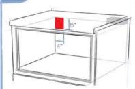
Place electrical outlet in upperback left side of opening. Electrical outlet can also be placed in an adjacent cabinet. Always check electrical codes for requirements. Proceed to Installation Instructions to install Drawer into cabinet.
