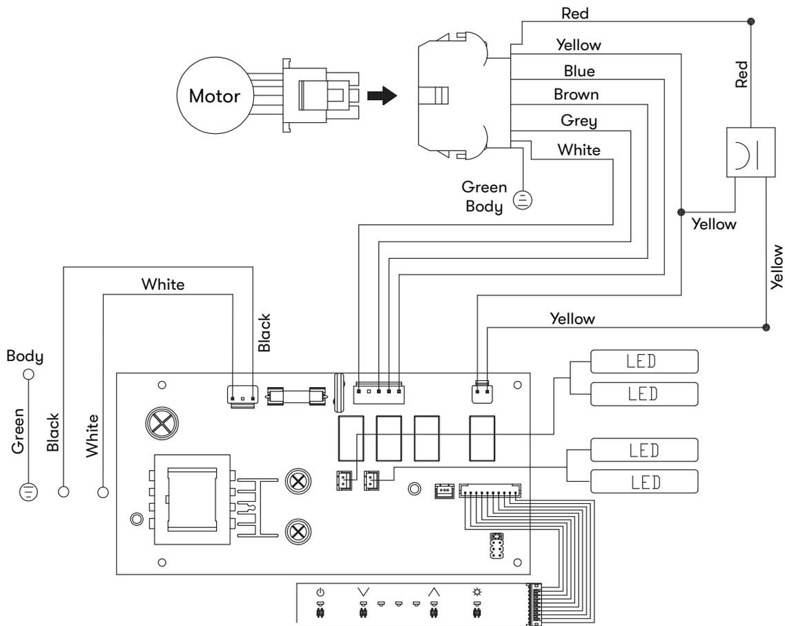
REMARKS: CONDENSER 12.5+12.5uF 250V AC FIT AC120V 60Hz
