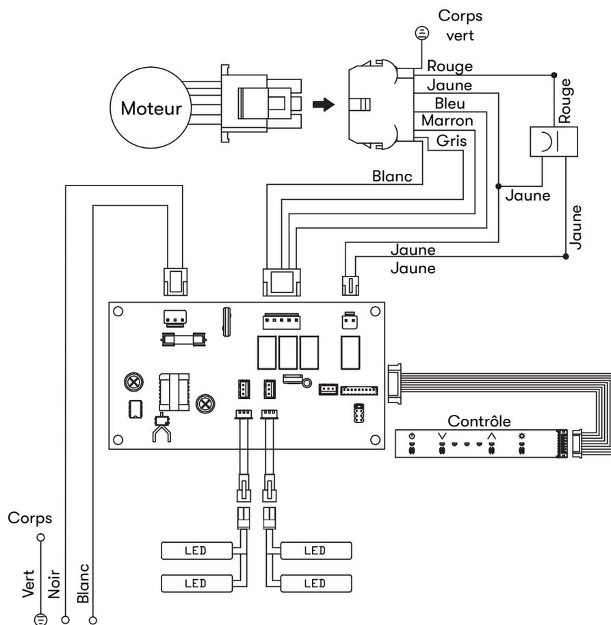
REMARQUES : CONDENSEUR 12.5+12.5uF 250V AC FIT AC120V 60Hz
