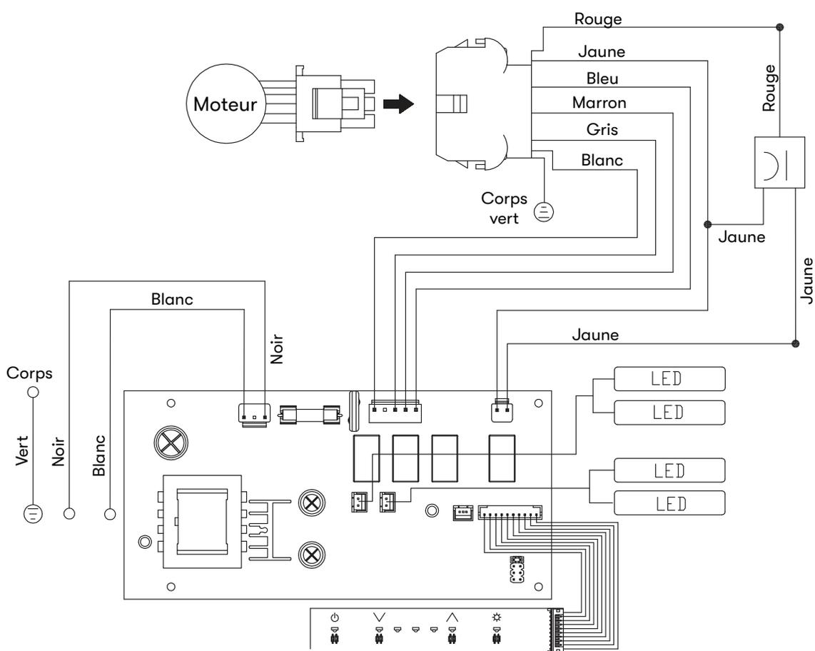
REMARQUES : CONDENSEUR 12.5+12.5uF 250V AC FIT AC120V 60Hz
