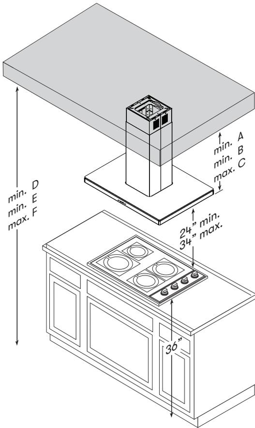
A minimum of 6" round duct must be used to maintain maximum air flow efficiency.
