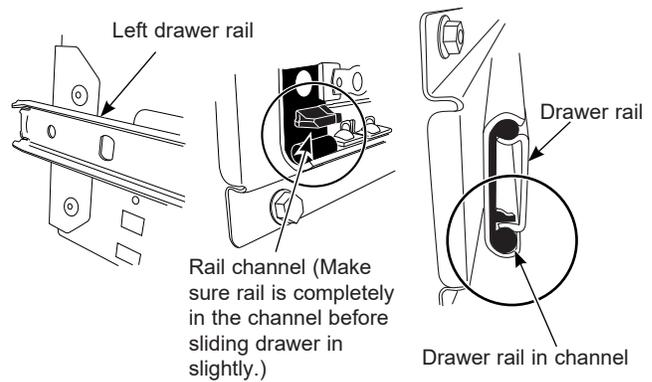
2. Place the right drawer rail inside the inner right rail guide channel at the top and slide it in slightly.
