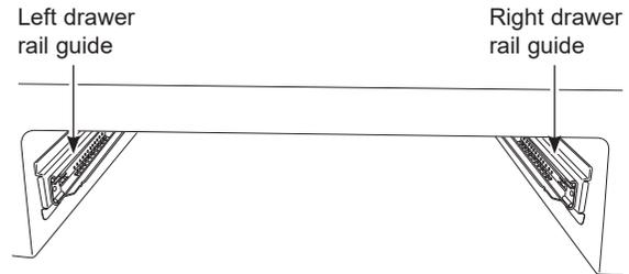
1. Rest the left drawer rail inside the inner left rail guide channel at the bottom and slide it in slightly.
