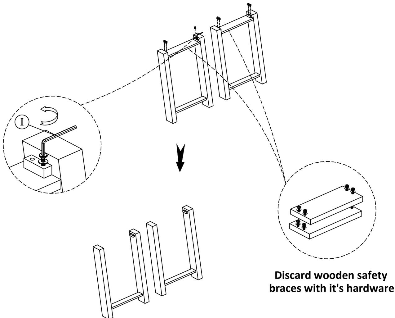
**Step 2 : Do not fully tighten the bolts**
