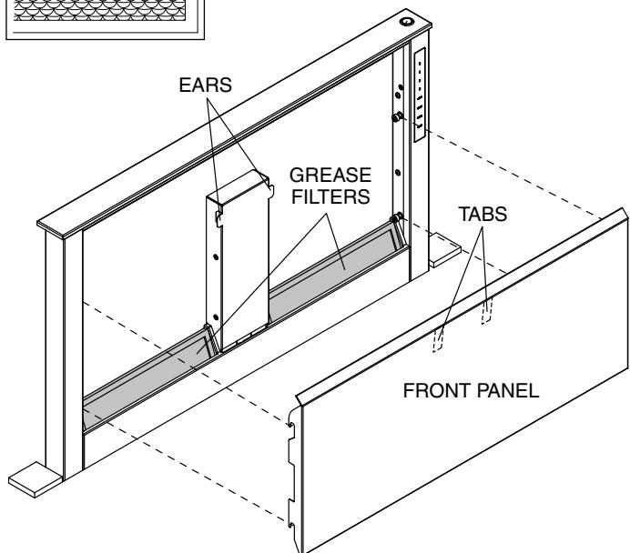
To remove the front panel, lift the panel up and pivot out at an angle. The panel can be removed fully.
