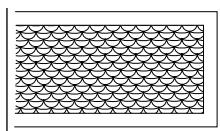
For best performance: Replace grease filters with half-moon openings facing out - and in orientation shown.
