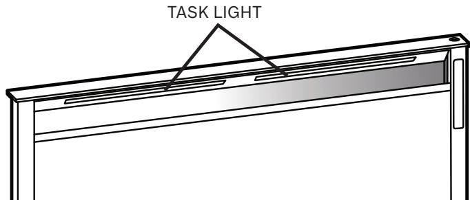
Touch and release the LIGHT icon on the control panel to control the light across the top of the hood.
