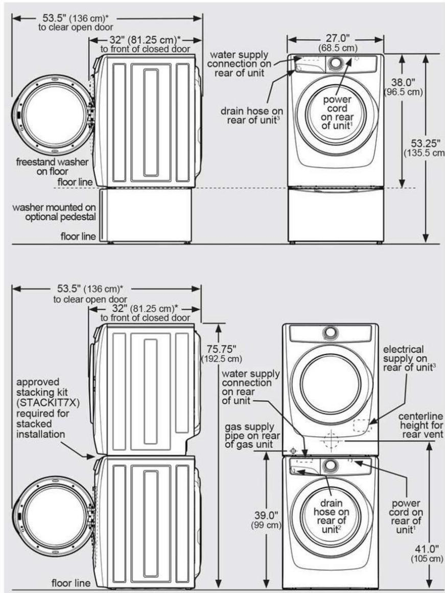
\*Connection of water inlet hose on steam dryer adds 3/4 in. (2 cm) to installation depth.
