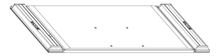
2. Place speaker rail assemblies on back of TV and align holes on rails to holes on back of the TV. Ensure center of Décor Fixed Mounting Rail is centered to width of TV.
