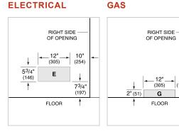
NOTE: Dimensions in parenthesis are in millimeters unless otherwise specified
