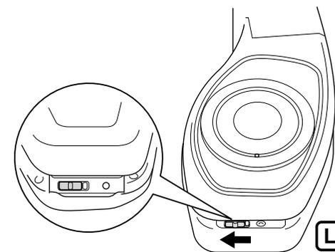
Turn the noise cancelling function toggle switch to on. When the switch is flipped, the blue LED indicator will flash two times.
