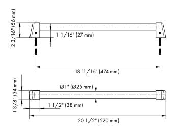
For Refrigerator Drawer models, use the included M5x20 to install the studs.
