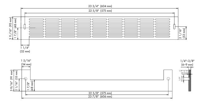
NOTE: When finishing the grill/plinth, be sure to stain front, back and all edges to prevent warping. Apply double-sided tape to the surrounding edges of the integrated grill/plinth as shown above. Remove the backing paper from the double-sided or hook and looptape. Carefully align the grill/plinth over the integrated grill/plinth and press into position.
