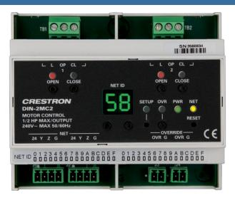
**OVERRIDE:** (2) 2-pin 3.5mm detachable terminal blocks, paralleled; Sensing input for external low-voltage contact closure; Activates override mode when a closure is present; Minimum Closure Rating: 10mA (per module) at 24 Volts
