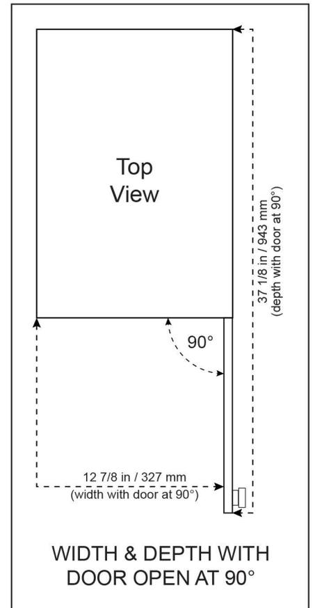
\*Please note: the unit depth with handle, when door is closed, is 24 7/8 in (632 mm)
