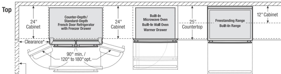
\*When installing French door refrigerator adjacent to wall, cabinet or another appliance that extends beyond front edge of unit, 20" minimum clearance recommended to allow for optimum 120° to 180° door swing, providing complete drawer/crisper access and removal. (Absolute 4-1/2" minimum clearance will ONLY allow for 90° door swing which will provide limited drawer/crisper access with restricted removal.)
