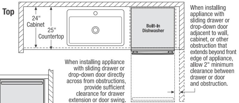
Use these dimensions and clearance instructions for planning purposes only. For detailed installation instructions, refer to installation guide, packed with product, or on the web at [frigidaire.com](http://frigidaire.com).
