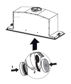
Attach each charcoal filter to the black grid on each side of the blower. Press the charcoal filter tightly to the black grid on the blower side and rotate the filter clockwise (towards the front of the insert hood) until it locks into place. Turn counterclockwise (towards the back of the insert hood) to remove.
