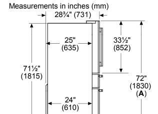
**A**: Add <sup>5</sup>/8" (17) with front leveling feet fully extended
