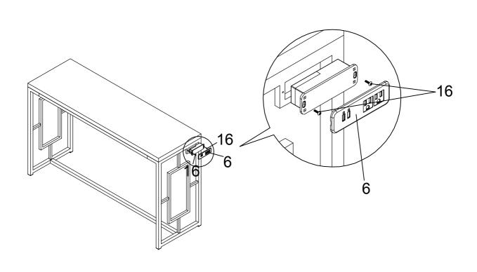
Step 3: Insert Power (6) into Bar Table Right Frame (3) using Power Bolt (16) as shown.
