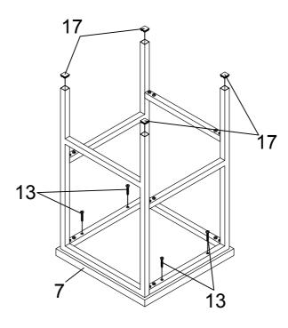
Step 6: 1. Attach the assemble in Step 5 to Chair Top Panel (7) using Medium Bolt (13) as shown.
