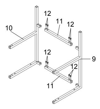
Step 4: Attach Chair Crossbar (11) to Chair Left Frame (9) and Chair Right Frame (10) using Short Bolt (12) as shown.
