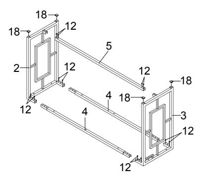
Step 1: 1. Insert Large Cap (18) into Bar Table Left Frame (2) and Bar Table Right Frame (3) as shown .
