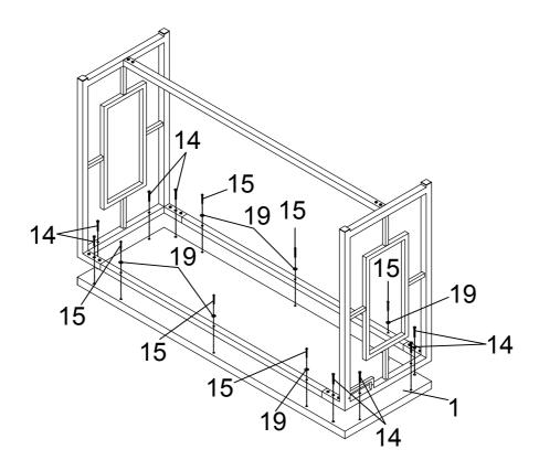
Step 2: 1. Attach the assemble in Step 1 to Bar Table Top Panel (1) using Long Bolt (14), Screw (15) and Washer (19) as shown.
