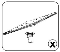
**WARNING:** Lower spray arm is metal; after removing the lower spray arm for maintenance and cleaning, do not disassemble the plastic part from the spray arm. This may cause injury due to possibility of sharp edge on the metal spray arm when plastic part is removed.
