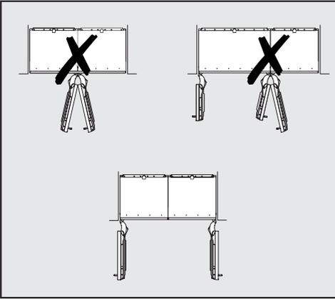
If the appliances are to be installed next to each other without a partition wall between them, they will need to be joined together with the side-by-side installation kit. In addition, you must install the side panel heater to prevent condensation from forming and any resulting damage.
