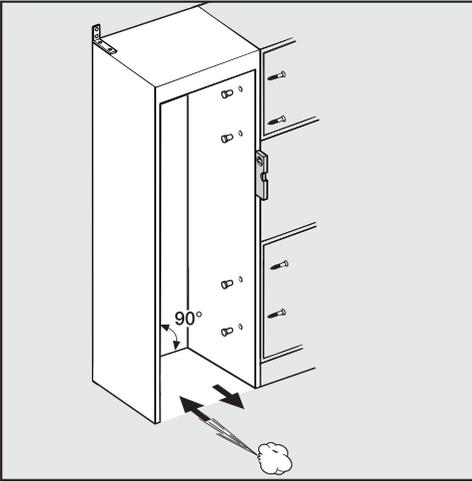
The building-in niche must be carefully aligned using a spirit level before the refrigeration appliance is installed. The niche corners must be at 90° angles to each other, otherwise the cabinet front will not sit straight on all 4 corners of the building-in niche.
