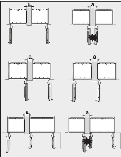
If the door hinges of the refrigeration appliances are next to each other, you must take into account the thickness of the cabinet fronts and door handles so that the appliance doors do not collide and become damaged if they are opened at the same time.
