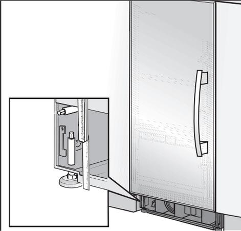
The adjustable feet at the front and back of the appliance can all be adjusted from the front of the appliance.
