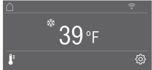
The sensor controls underneath the temperature display can be **selected** directly by touch; the symbols and text in or above the temperature display can only be **displayed**.
