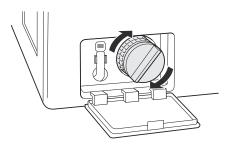
**8** Close the drain pump filter cover.
