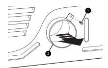
Press the tabs on the knockout 3 and carefully remove the knockout for the desired vent opening. (Right-side venting is not available on gas models.) Press the adapter duct **4** onto the blower housing and secure to the base of the dryer as shown.
