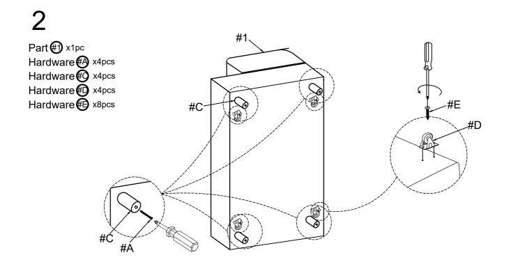
Align legs (#C) and wheels (#D) to the bottom of loveseat (#1), then secure by using screws (#E). There will be no pre-drilled holes on the bottom of the loveseat (#1).
