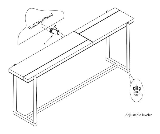
Adjust levelers if needed, to level case on uneven floor
