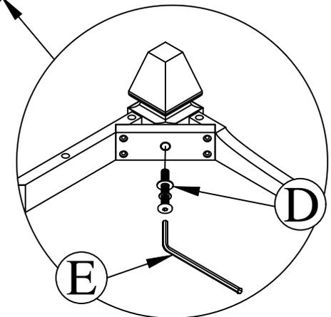
NOTE: MUST TIGHTEN SCREW PERIODICALLY. WITH USE SCREWS WILL BECOME LOOSE CHECK TIGHT OF ALL SCREWS EVERY 6-8 WEEKS.
