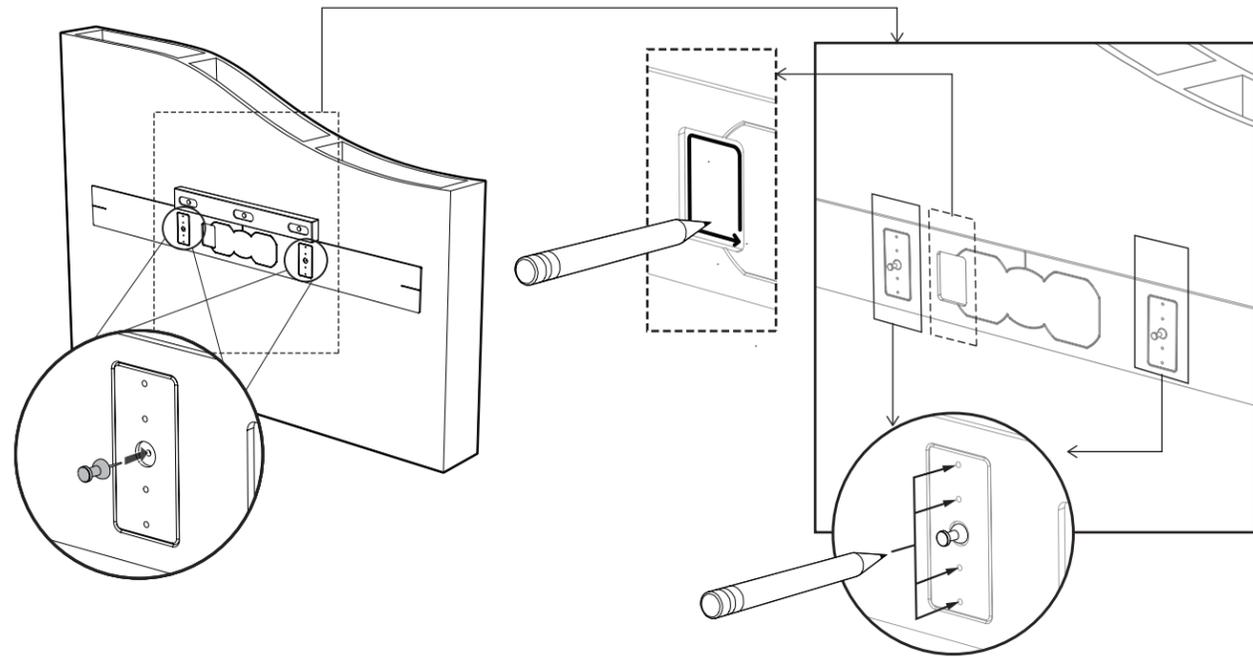
**1** Use level and included pushpins to secure Mounting Template to wall in desired mounting location.
