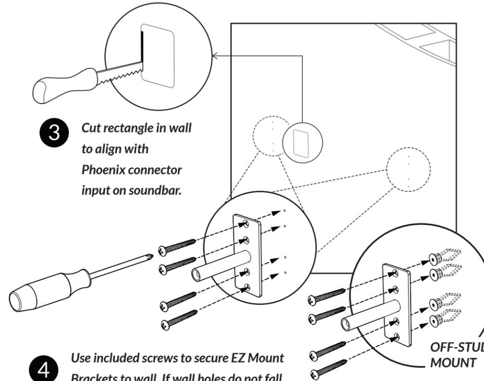
**3** Cut rectangle in wall to align with Phoenix connector input on soundbar.
