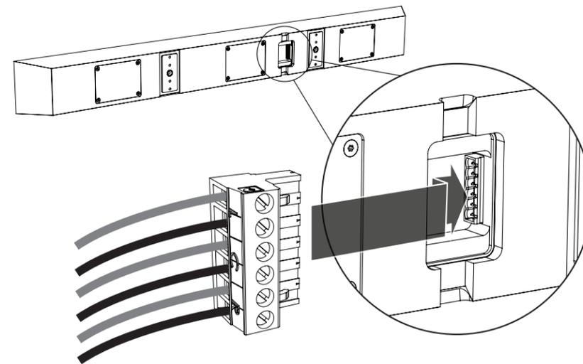
**7** Insert male Phoenix connector into female Phoenix receptacle in back of soundbar until it clicks firmly into place. To remove, pull firmly on male Phoenix connector.
