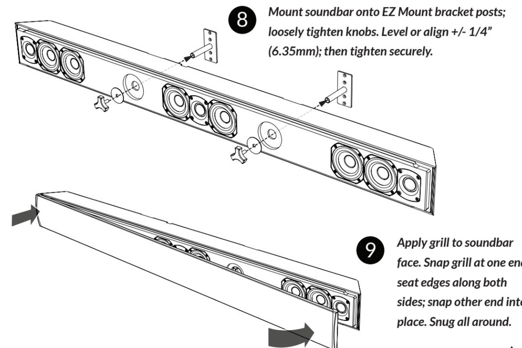
**8** Mount soundbar onto EZ Mount bracket posts; loosely tighten knobs. Level or align +/- 1/4" (6.35mm); then tighten securely.
