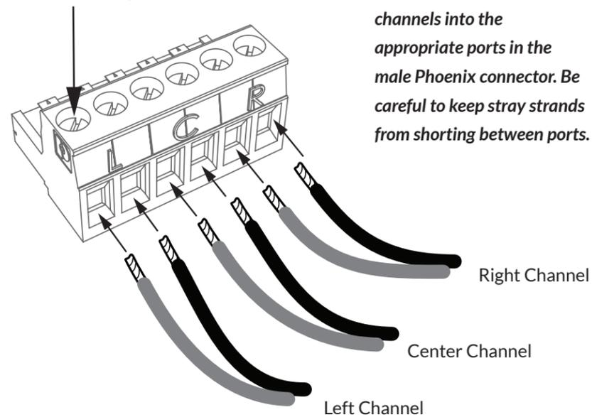
**6** Depending on configuration, insert wires from available channels into the appropriate ports in the male Phoenix connector. Be careful to keep stray strands from shorting between ports.
