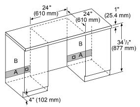
A٠ Recommended area for installation connection - a  $2^{1/2}$ " (63 mm) diameter hole is recommended. Location of power cord at base of the appliance. 5<sup>1</sup>/8" А Α
