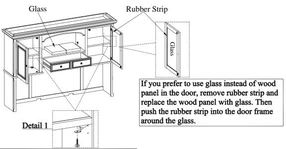
When you prefer to adjust the location of shelf, take off screws and reinsert the shelf brackets into the holes. Then place the shelf on and re-securing it.
