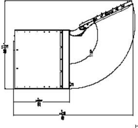
Max clearance required for opened door is 49-3/4'' when opened to  $90^{\circ*}$  (dimensions shown are without door overlay installed.)
