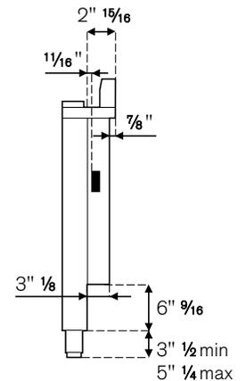
Bertazzoni recommends to operate the appliance after it has been installed in a cabinet. The kitchen cabinets shall be made of materials capable of withstanding temperatures at least 117°F (65°C) above room temperature in order to avoid possible damage to the cabinets during oven usage. For further installation instructions refer to the installation manual.
