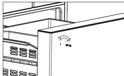
2. Screw the locating bolt into the bolt hole of the door body and secure it.
