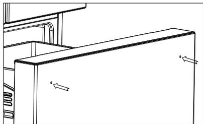
1. Before the refrigerator door handle is installed (note: the anchor bolts of the handle are in the accessory bag, and all steps should be performed at the right and left two mounting positions simultaneously).
