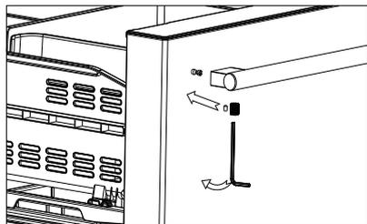
3. Loosen the locking screw inside the handle part with a hexagonal wrench first, then align the handle with the positioning bolt and insert it into the positioning bolt (note: the handle locking screw is installed facing down).
