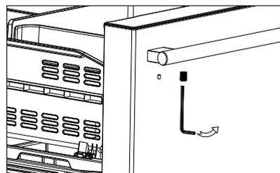
4. Wait until the handle fits perfectly with the door body, and then use a hexagonal wrench to tighten the locking screw inside the handle part.
