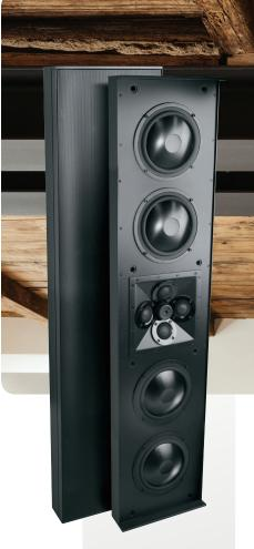
Size40 h x 9.75 w x 2.739" d (in)<br/>1016 h x 248 w x 79.5 d (mm)Freq Response70Hz-40kHz±3dB<br/>ImpedanceImpedance4 ohms<br/>96dB 2.83V /1mPower req.25 -200 watts<br/>VooferWoofer(4) 6.5" (165mm) Aluminum<br/>Utra-SlimTweeter(4) 1" (25mm) Beryllium Dome<br/>Through hole (Optional Brackets)<br/>FinishesFinishesGloss White, Satin Black,<br/>or Custom
