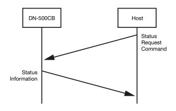
3. Status information automatically sent to the host when a change is made from DN-500CB
