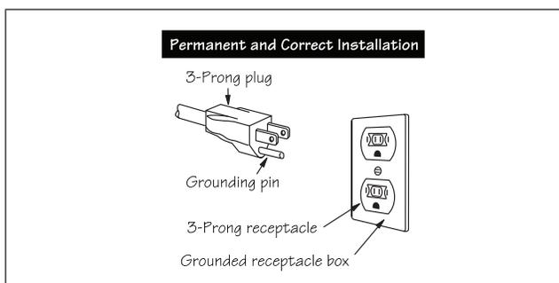
**WARNING** - Improper use of the grounding plug can result in a risk of electric shock. Do not use an extension cord. If the power supply cord is too short, have a qualified electrician or serviceperson install an outlet near the appliance.
