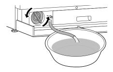
**5** Clean the pump filter and opening.
