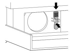
**7** Insert the drain pump filter and twist it clockwise.
