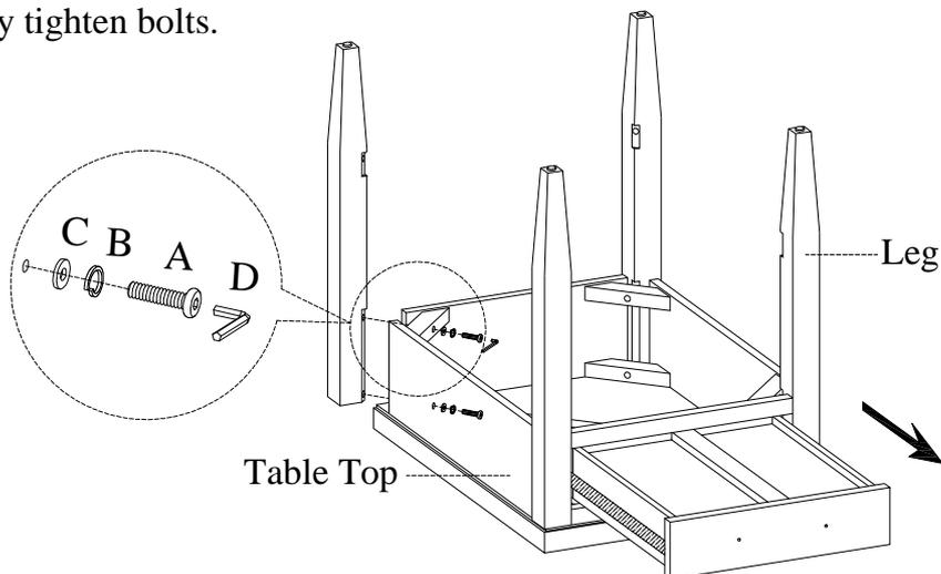
**STEP 2:** Attach the bottom shelf to the legs by using 4 bolts (A), lock washers(B) and flat washers(C). Completely tighten all bolts. Push the drawer back. Turn the assembled table to the upright position.
