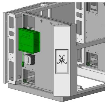
13. Mount the lift-off panel on the left side of the suite. There are pins on either side for locating. The louvers located on these side panels are needed for ventilation and must not be blocked. If this lift-off panel does not install/remove easily, you may need to adjust the corner assembly to accommodate (see Step 7).
