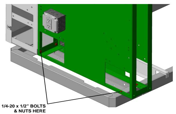
2. Install remaining support walls as you did in step 1. Each wall is numbered and has a corresponding number on the curb and/or rear wall for ease of locating. (12 foot Outdoor Living Suite with Bar shown).
