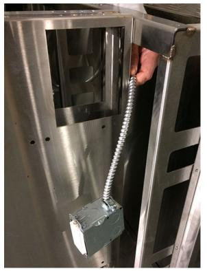
Line up and install 4 each #10 screws as shown here.
