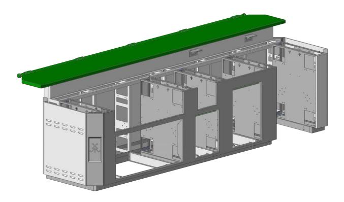
4. While an assistant is holding the bar top in place, reach underneath and secure the top with 1/2'' nuts and lock-washers provided. Then secure the large back panels with  $1/4-20 \times 1/2''$  long bolts and flat washers.
