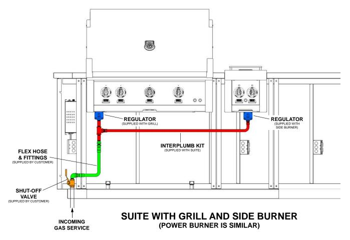
2. The remaining gas connections shown above must be completed by the qualified plumber or professional outdoor appliance installer. See reference photo on the next page for typical flex hose and shut-off valve location. Flex hose, shut-off valve, and misc. fittings must be provided by the homeowner and installed by the qualified plumber or professional outdoor appliance installer. The gas regulator is supplied with the grill & side burner (or power burner).
