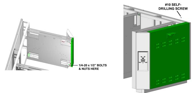
Install large front panel as shown using 1/4-20 x 1/2" long hex bolts and hex nuts where needed. (8 foot Outdoor Living Suite shown)
