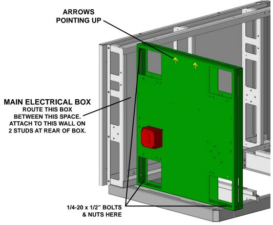
5. Install remaining support walls as you did in step 4. Each wall is numbered and has a corresponding number on the curb and/or rear wall for ease of locating. (8 foot Outdoor Living Suite shown) Do not fully tighten bolts yet. Note all arrows are pointing up.
