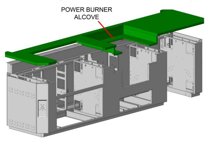
2. There are four (4) #8-32 x 3/8" flathead countersunk screws which attach the alcove to the front panel.
