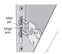
Figure 18: Replacement and location of hinge arm and roller pin
