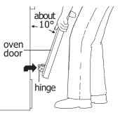
Figure 17: Holding door for removal
